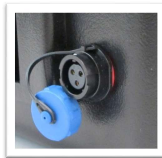
Laden / Charge Weipu IP67
